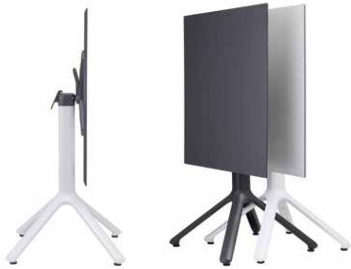
**Mesa fija y plegable** con columna cuadrada con esquinas biseladas en aluminio y base de 4 pies. Tapa compact laminado. Uso interior o exterior cubierto. Die cast aluminium four feet base. Square aluminium column with rounded corners. Die cast aluminium brackets for fastenin to top. Folding mechanism with handle for easier alignment of several tables. Whit 4 ajustable feet.
